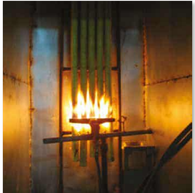
Cable samples in the harnessed cable burning test.
