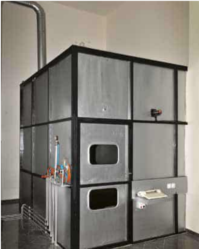
Smoke density testing cabin.
