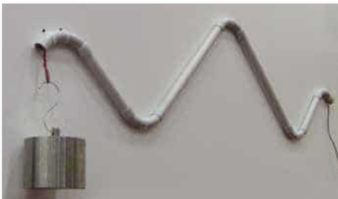
A cable sample in the slickness test.
