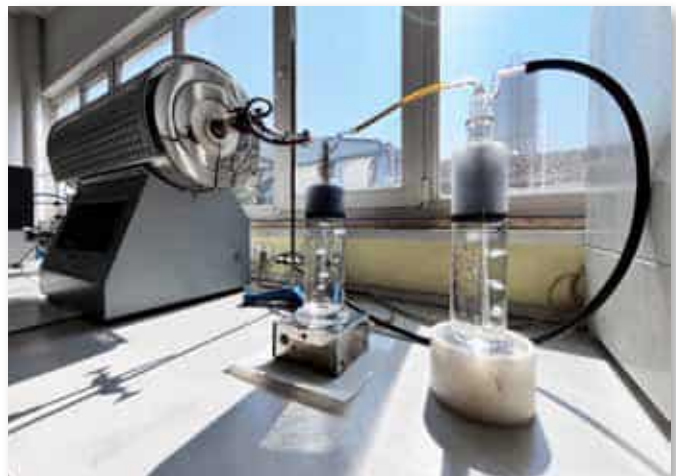
The halogen amount is measured by absorption of the burning gas into water.
