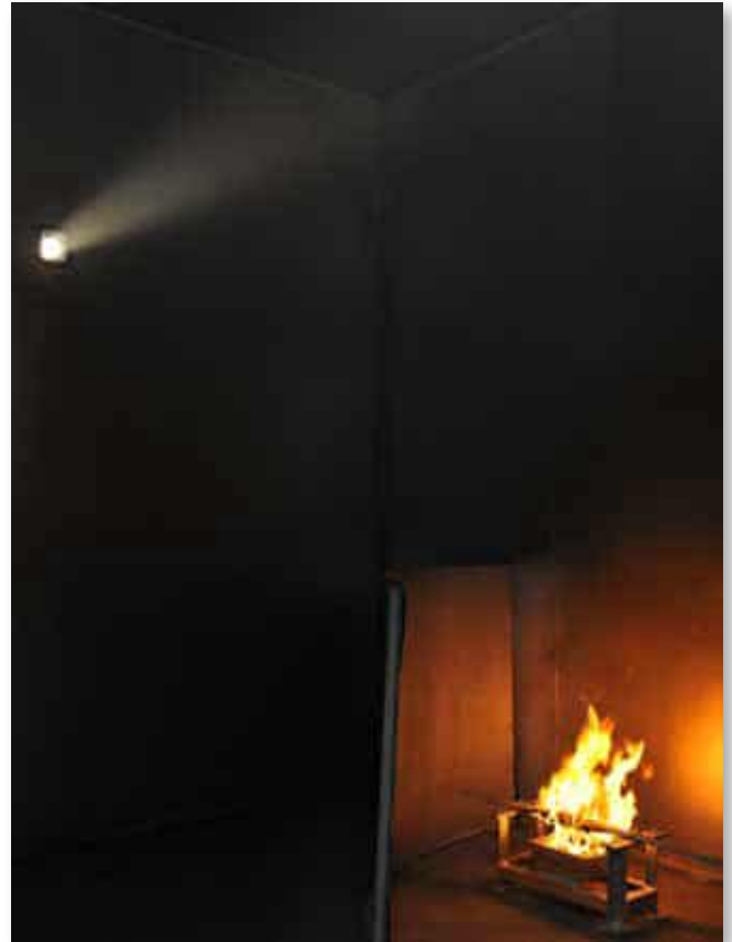
A cable sample in the smoke density test.
