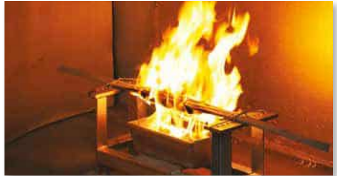
In smoke density tests, fuel should be used as specified in the standards.
