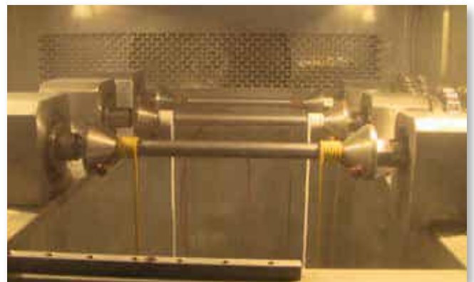
Cable samples in a cyclic strength test.
