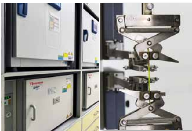
Ovens used for aging tests.
