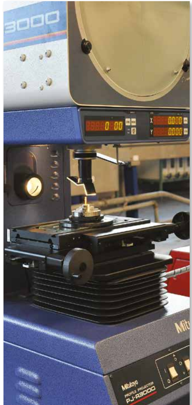
Geometric measurements are made using a profile projector.
