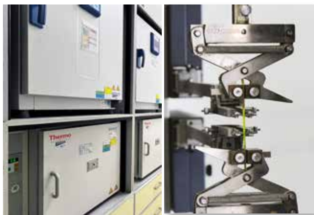
Ovens used for aging tests.
