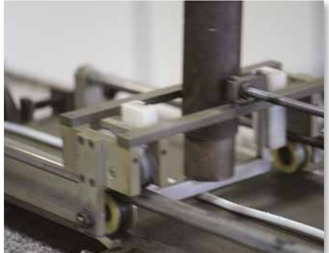
A cable sample in the abrasion test.
