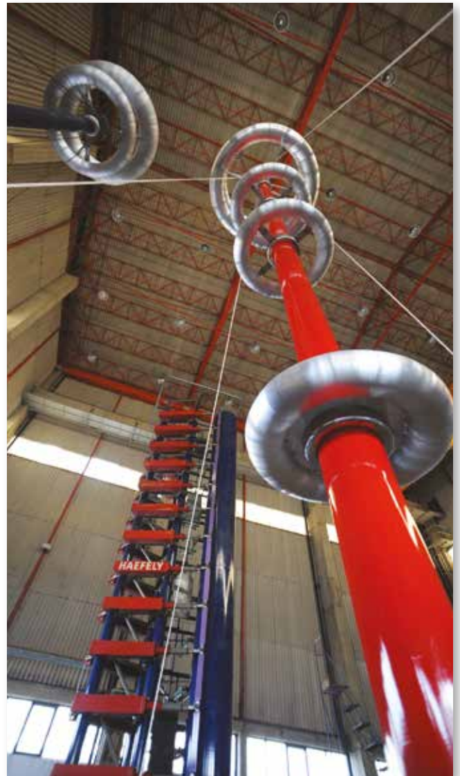
Lightning impulse generator voltage divider.
