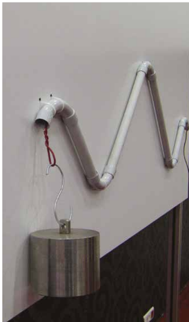
Slippery cables can move through ducts even with small amount of force.
