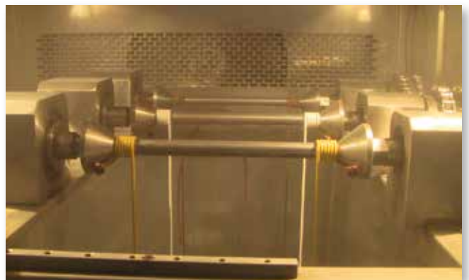
Cable samples in a cyclic strength test.
