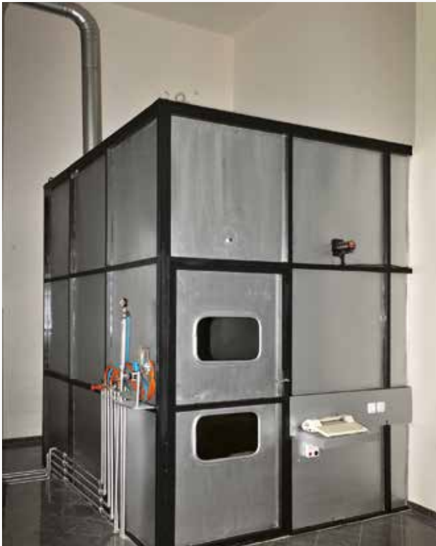
Smoke density testing cabin.
