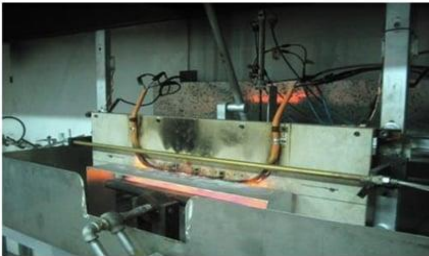
Figure 4: EN 50200 Test System
